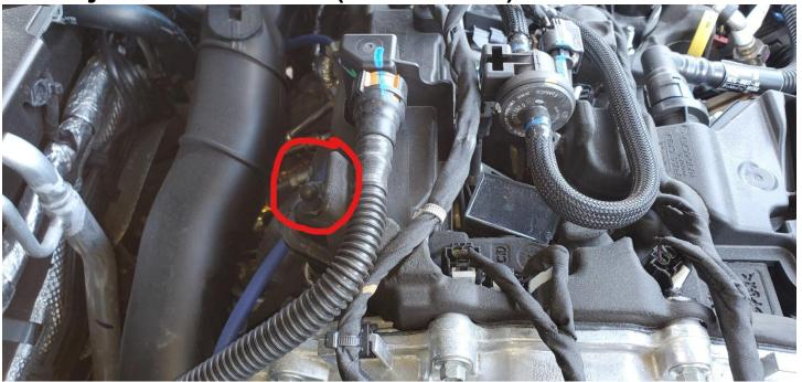
Alright this is where it gets a little tricky. The bracket circled in red (Top right of Engine) only purpose is to hold the wire tubes that are zip tied to it. This bracket has to be removed due to interfering with the engine cover's next ball stud which is under this bracket.
