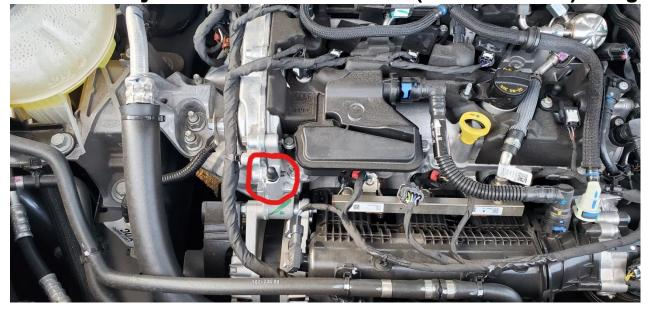
Going straight back towards the wall of your engine bay towards the Inside of your vehicle from the first ball stud installed is where your second ball stud (AA5Z 6N958-A) will be installed.
