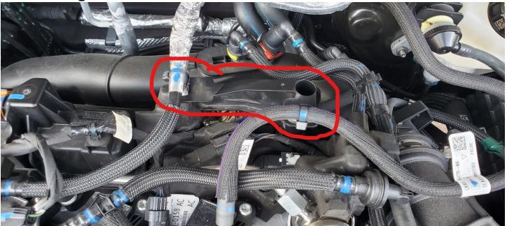
This bracket is removed by first cutting the zip tie off the tubes (careful not to snip the tube). Then moving the tubes a little to the side out the brackets way, grab the bracket underneath by the circle opening and pull straight up with a little force.
