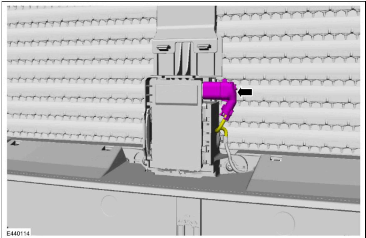
3. Release the clip and remove the CCM from the bracket.
